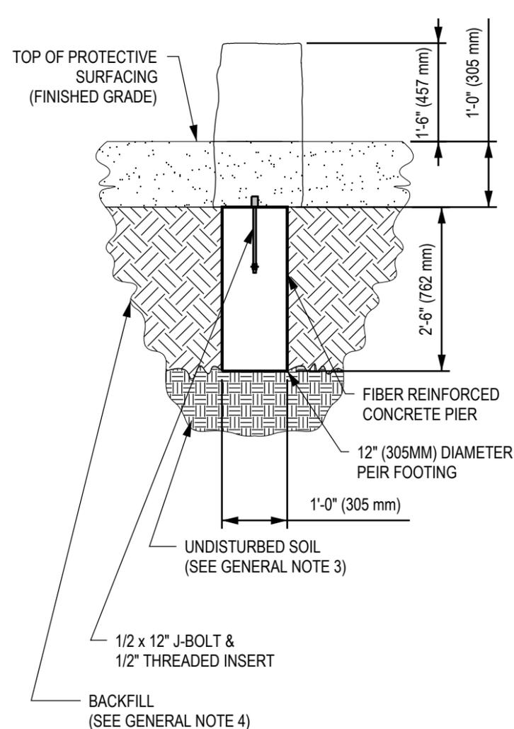
FOUNDATION DETAIL - ELEVATION VIEW
