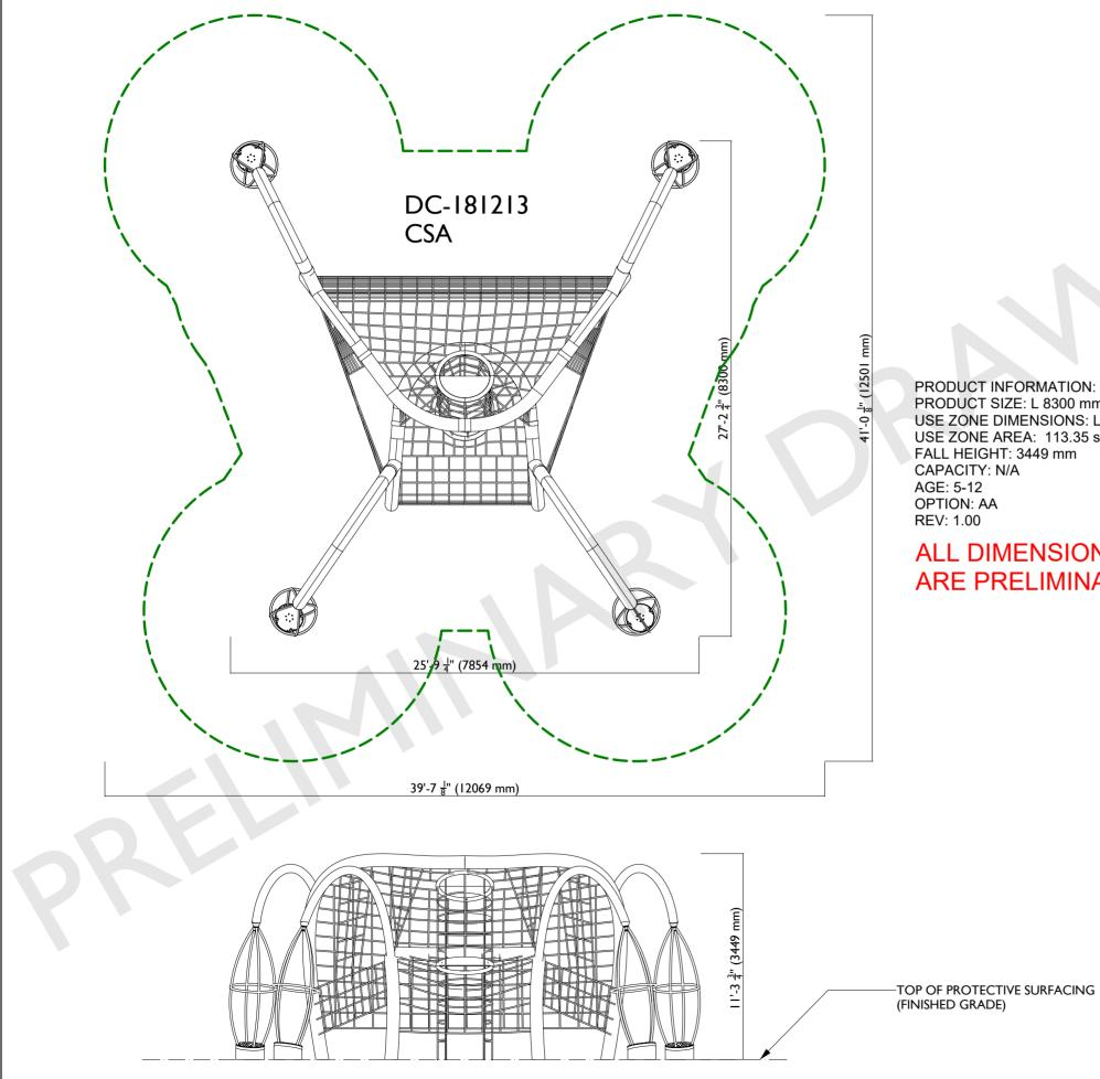
PRODUCT SIZE: L 8300 mm x W 7854 mm x H 3449 mm USE ZONE DIMENSIONS: L 12501 mm x W 12069 mm USE ZONE AREA: 113.35 sq m FALL HEIGHT: 3449 mm CAPACITY: N/A AGE: 5-12 OPTION: AA
